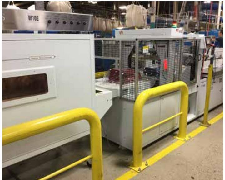
interviewed associate with Felins. The system transfers finished bundles from ironer and dry fold equipment via conveyors to the auto-wrapping mechanism. The system adapts to the plant layout via straight and cornering transfer conveyors, a traffic control system, a wrapper (aka bagger) and a shrink tunnel.
